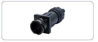
Sturdy depot plug with two auxiliary contacts, they close lagging the circuit when inserting and open leading it when removing.
