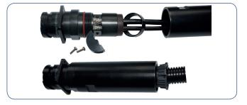
Backshell, fully rubber covered as protection against sandblast and abrasions, including a full receptacle cover. With integrated cable strain relieve and 360° shield connection against EMI impacts.
